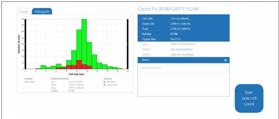
Figure 5. The size histograms of the live and dead cells are displayed in one chart. The histograms can be gated by moving the black bars on the left and right side of the chart.
