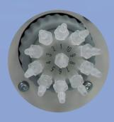
Pump distributor for 10 connections, controlled via the respective staining programm
