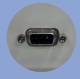
RS232 printer connection for optional operating of a thermal printer
