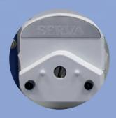
Peristaltic pump for quick and accurate filling/emptying of the staining dish
