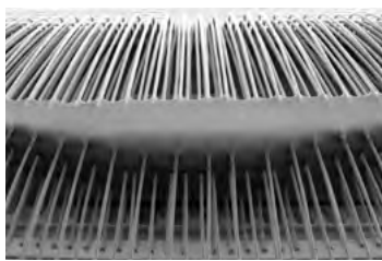
SEM of NoSWEEP™ Ring-lock dispense method on the same quad tier copper wire bonded device.
