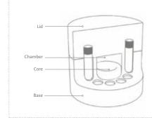
Corning CoolCell LX uses a combination of uniform-density cross-linked polyethylene foam, a solid state core, and radial vial symmetry to create freezing profiles that are consistent and reproducible. The low heat content also ensures that CoolCell LX containers will rapidly return to room temperature when removed from the freezer.
