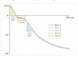
**Performance test:** A temperature probe was placed into a 2.0 mL cryogenic vial containing 1.0 mL of water and the tube was inserted into a room temperature Corning CoolCell. The CoolCell was placed into a -80°C freezer and the temperature rate and profile was recorded over a 3-hour period. The test was repeated 5 consecutive times.
